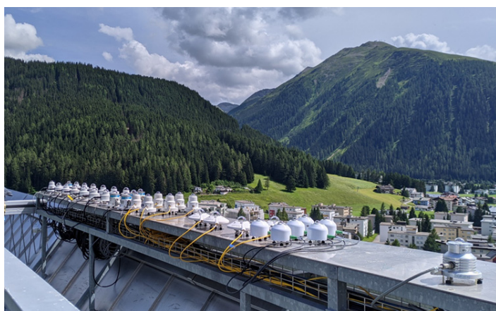
Figure 7. Solar UV filter radiometers on the measurement platform of PMOD/WRC
