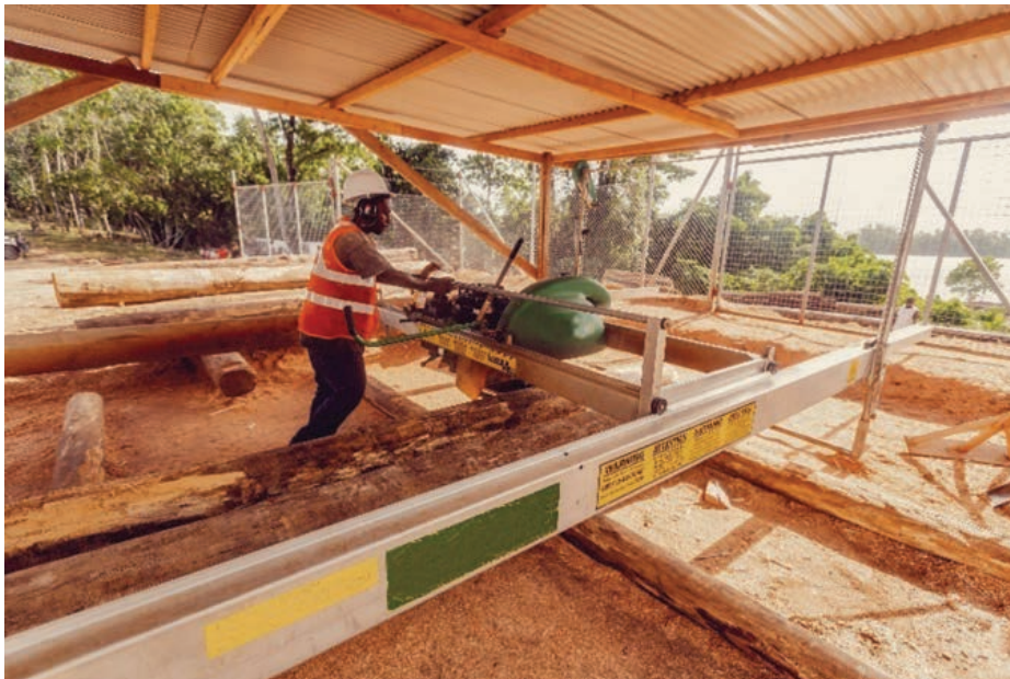
Kolombangara Forest Products Ltd. pallet plant staff demonstrate the construction of pallets from logs through to the finished product.
