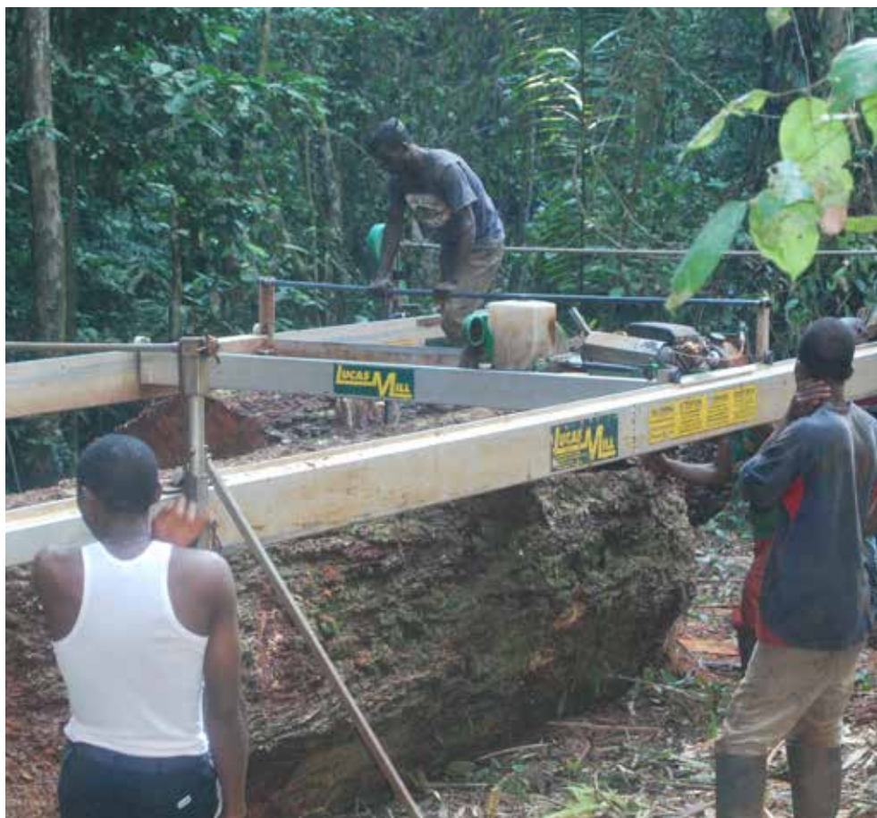
PHOTO 37 On-site conversion (a form of small-scale sawmilling): a challenging/dangerous work environment.
