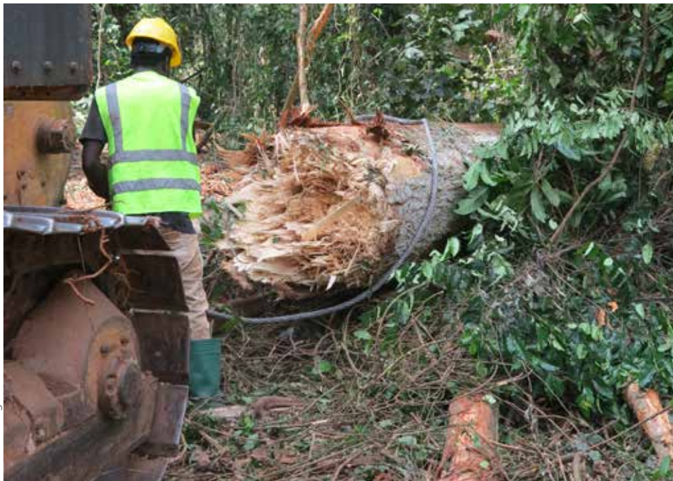
PHOTO 10 A choker setter (hookman) in action
