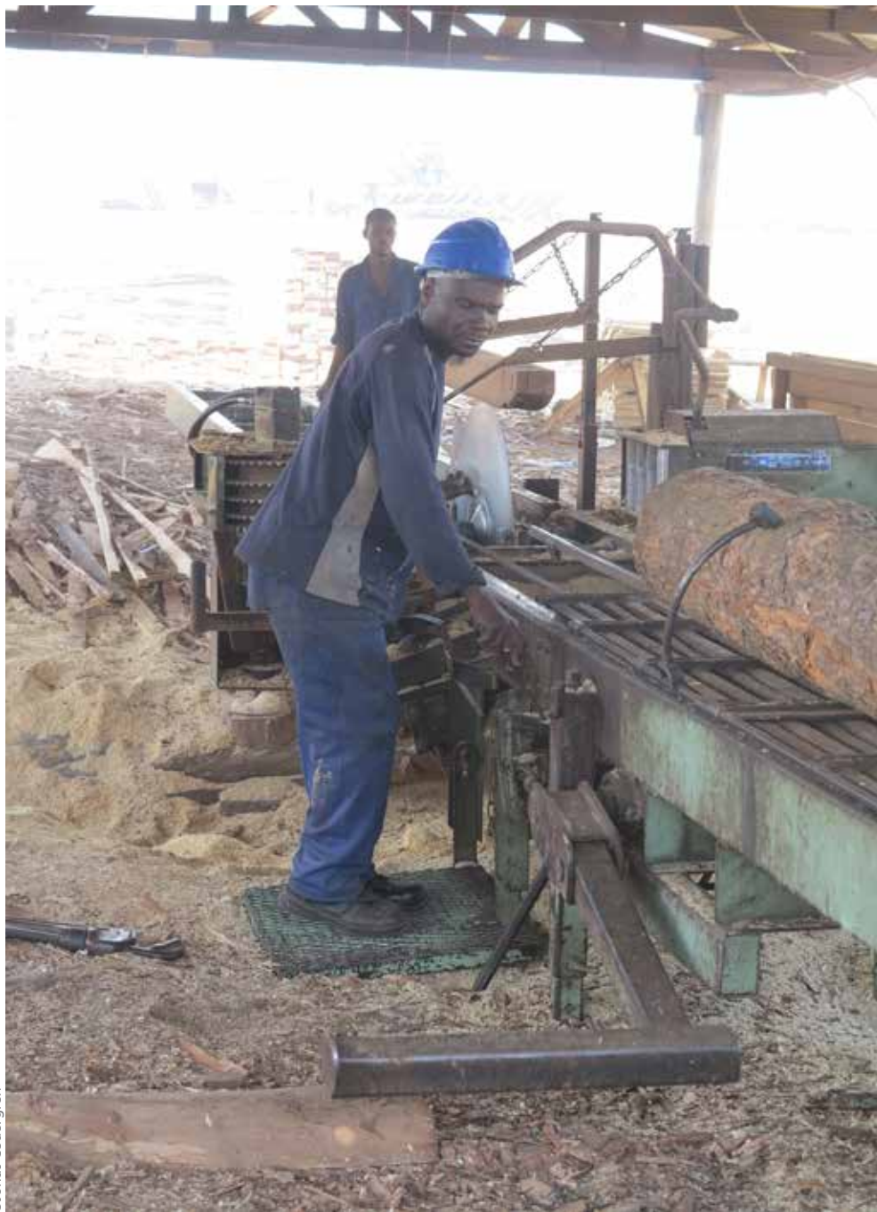
PHOTO 36 Circular saw, unguarded
